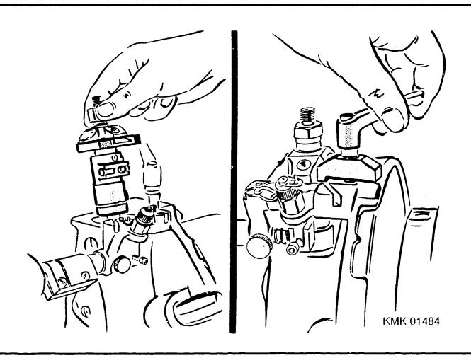
Screw prescribed test-pressure line to fuel-injection pump.
